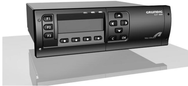
Figure 3.4 Hybrid GNSS/CN/DSRC Toll Collect OBU designed specifically for Toll Collect to be used in HGVS for in-dash mounting. (Courtesy of Efkon Mobility, Delphi Grundig, and Toll Collect.)
